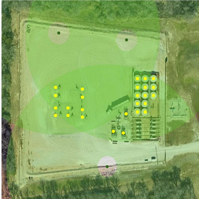
Figure 4 Visualization of the Nubo monitor operational range. Green dots indicate locations of Nubo devices, yellow dots indicate potential emission sources. The shaded green circles show the operating range of each Nubo monitor covering all potential emission sources.
